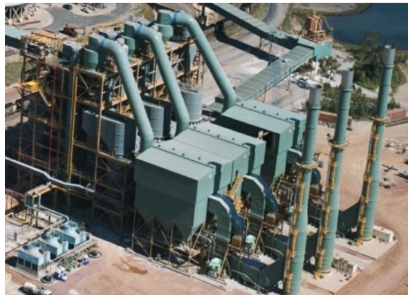
Figure 3. GSC with HAL and FBC, without HV QAL, Australia- 3 X 4500 TPD GSC Unit.
