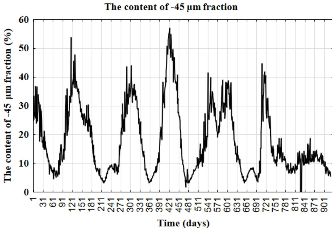
**Figure 2. The content of -45  $\mu\text{m}$  aluminum hydroxide fraction in the last precipitator.**
