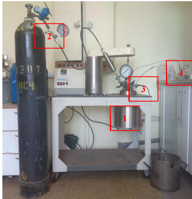
Figure 1. Autoclave installation for simulation of processes of preliminary desilication, digestion, dilution and post-desilication in the flashing circuit.
