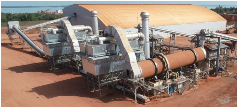
Figure 11. Dry bauxite storage and two dryers at the Dian-Dian mine.
