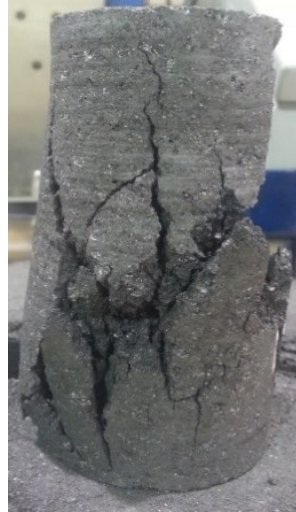
Figure 8. Ductile rupture obtained at 200 °C, 300 °C and 400 °C.
