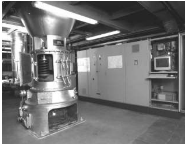
Figure 2. EM 17-525 Test Mill with Control System
