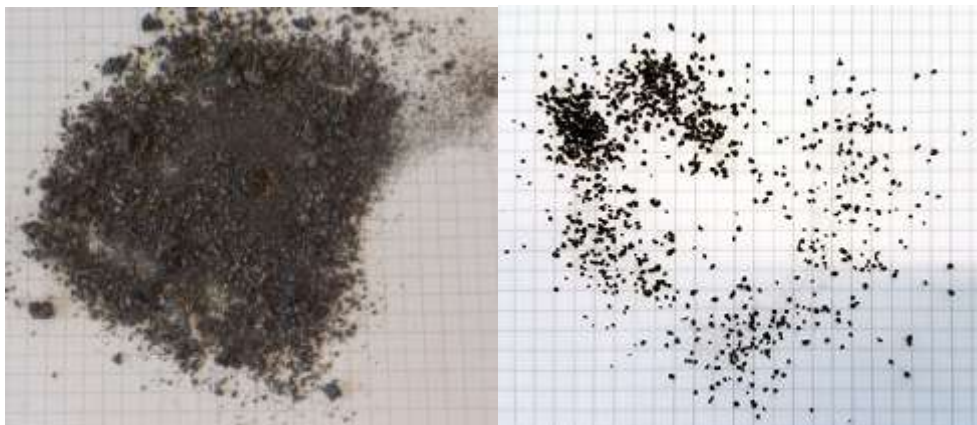
Figure 3. Mill feed - left: standard with natural size distribution < 10 mm right: feed for super fine grinding mono-size of approx. 1mm
