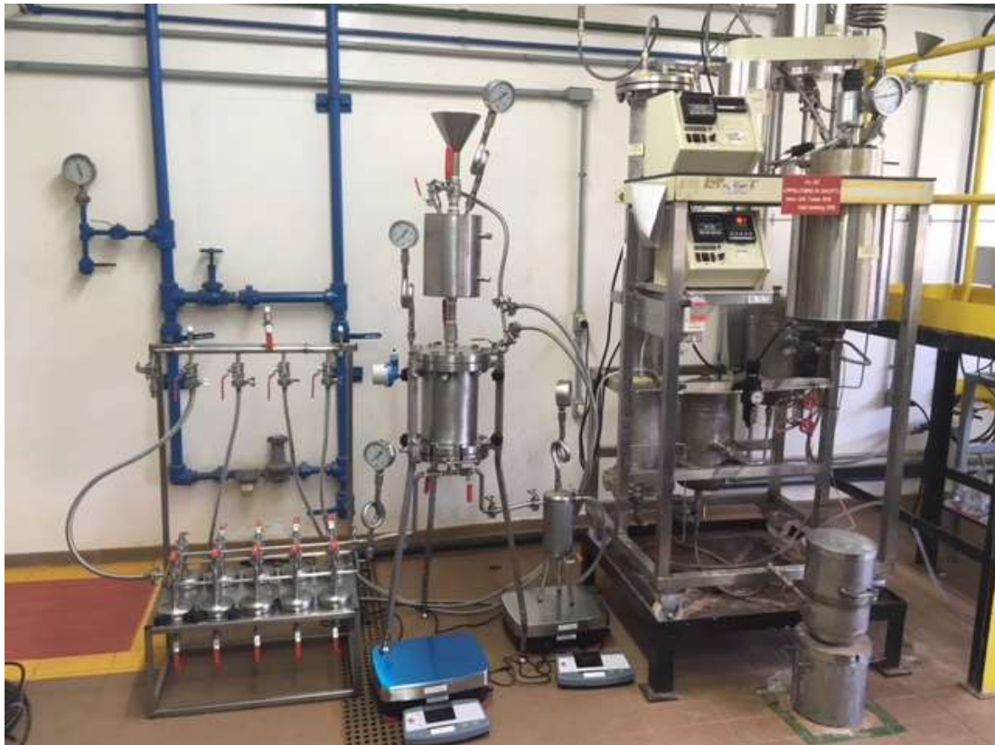
Figure 6. Autoclave apparatus (right) and pressure filter (left) in the B&A R&D laboratory.
