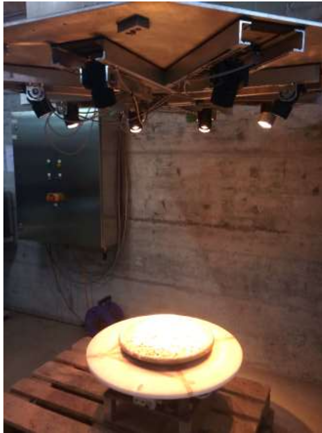
Figure 5. Calibration setup: NIR detector and sources.
