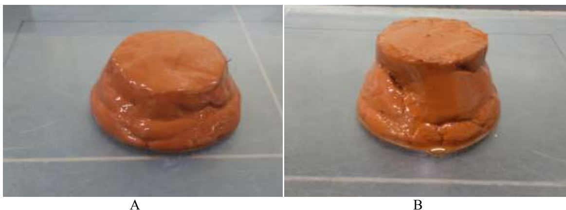
Figure 8. Slump test for the sediment formed with 30 g/t of AC 662 but varying the MF LT7990 dosage. (A) without MF LT7990; (B) 60 g/t of MF LT7990.
