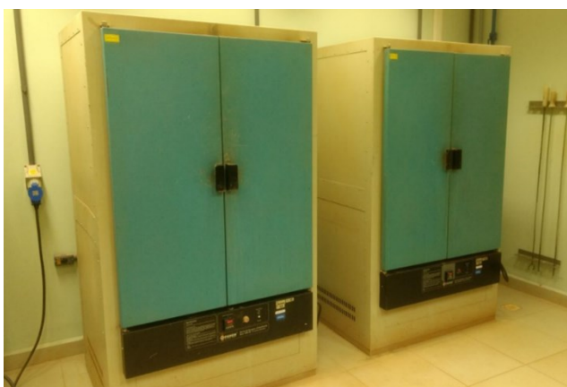
Figure 1. Hot air blower dryers.
