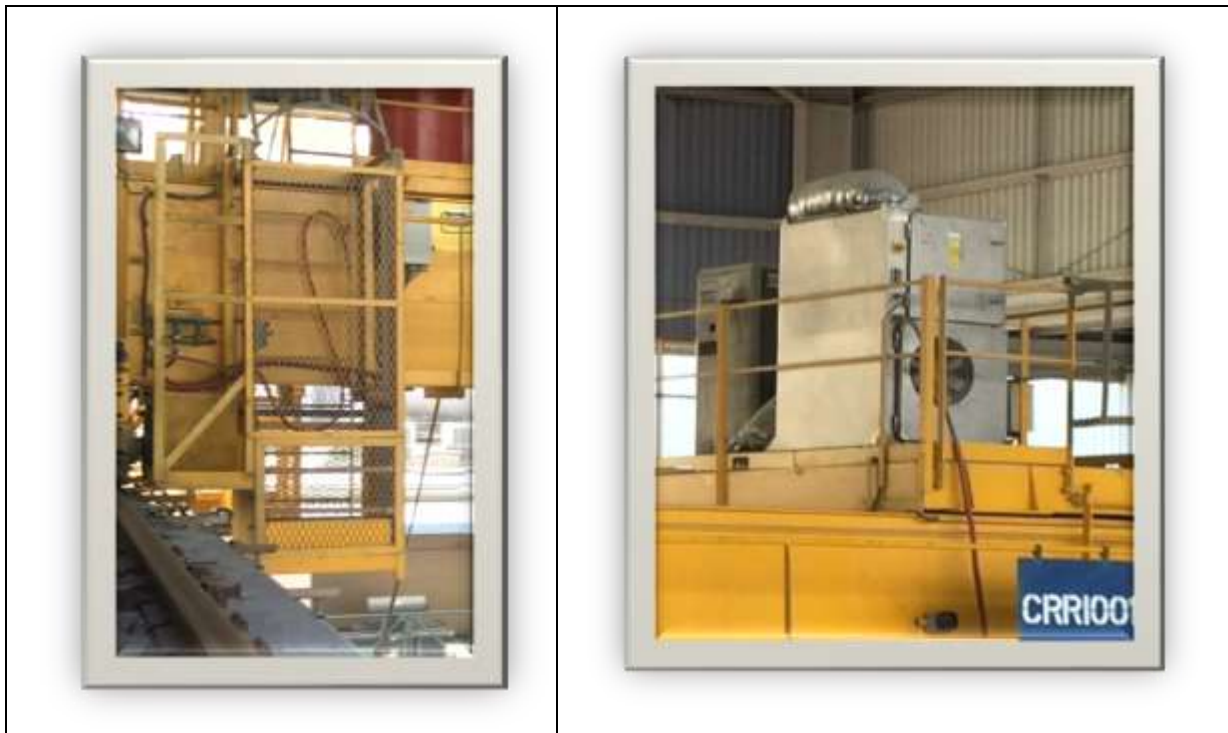
Figure 5. Left: man-carrying baskets, Right: air conditioning system.
