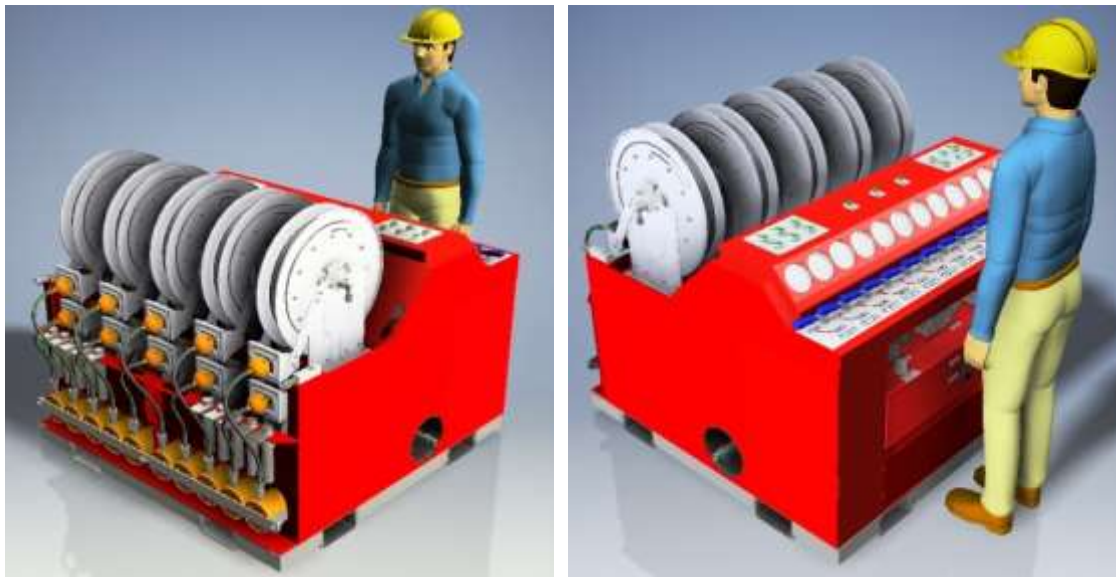
Figure 6. New hydraulic wedge puller. Left: back view, Right: front view.
