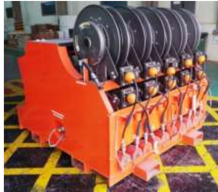
Figure 7. Wedge puller hydraulic unit with retractable reels.
