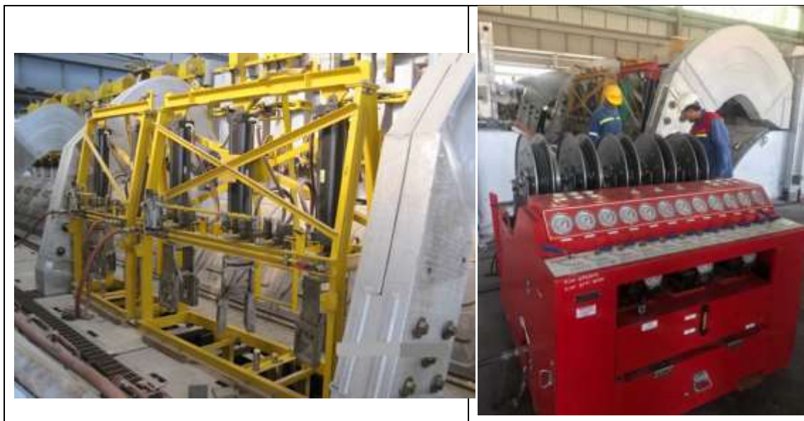
Figure 2. Wedge extraction system. Left: wedge extractor (A-frame). Right: wedge puller hydraulic unit (front) and wedge extractor installed for action. On the reels are the hoses that connect the two units and provide hydraulic oil to extraction jacks.
