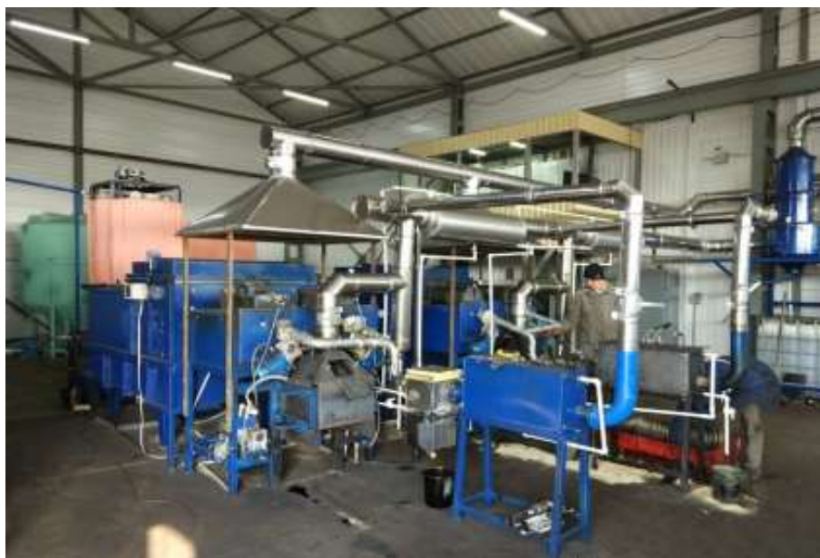
Figure 10. Pilot plant for production of extractive pitch.
