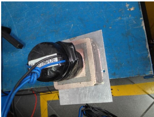
Figure 9. Electrode contacts and connections to the meter at EGA: for epoxy grout (left) and for ISOVAL® (right).
