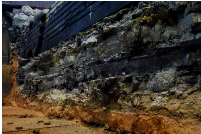
Figure 5. CBA cell lining cross section – Cell 1639 autopsy.
