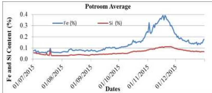
Figure 6. Iron and silicon concentration in the metal.
