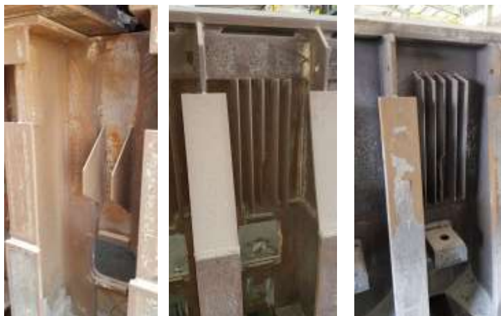
Figure 4. Comparison between Generation 1 (left), Generation 1 Modified (middle) and Generation 2 shells.
