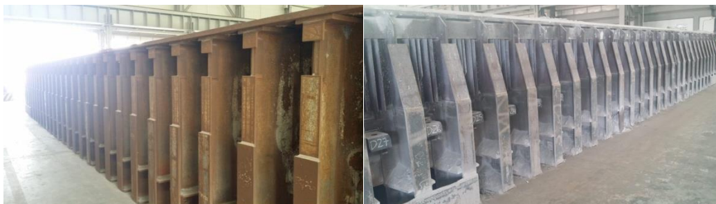
Figure 3. Potshell modification for more heat loss.
