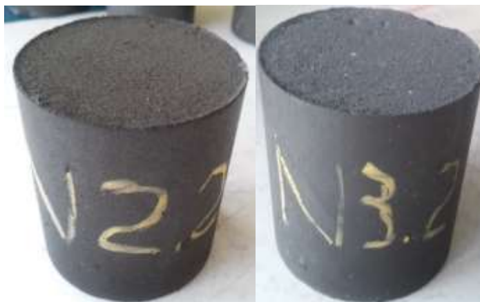
Figure 4. Aspect of cements C (on the left) and S (on the right) with a water to cement ratio of 0.4, and a content of graphite powder B of 50 %, after pressing under 10 kN.
