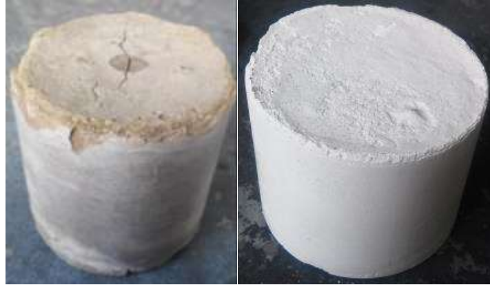
Figure 2. Aspect of cements C (on the left) and S (on the right) with a water to cement ratio of 0.4, and after 24 hours inside a plastic mold of 60 mm diameter.
