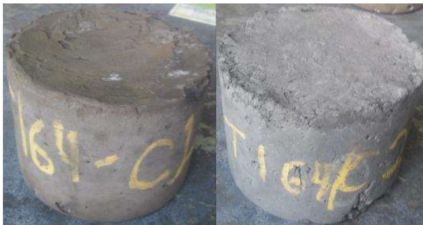
Figure 3. Aspect of cements C (on the left) and S (on the right) with a water to cement ratio of 0.4, and a content of graphite powder B of 25 %.
