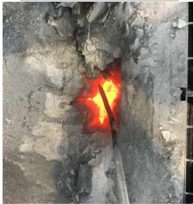
Figure 2. Electrode for anode voltage drop measurements.
