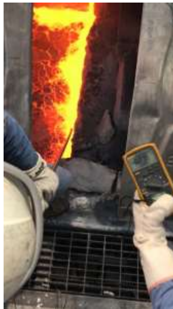
Figure 12. Measurement of anode voltage drop in point 3.
