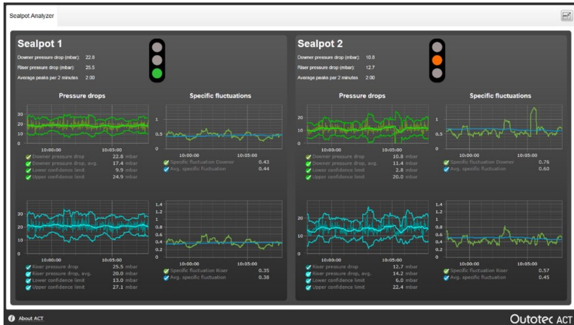
Figure 2. Seal pot operational monitoring system.
