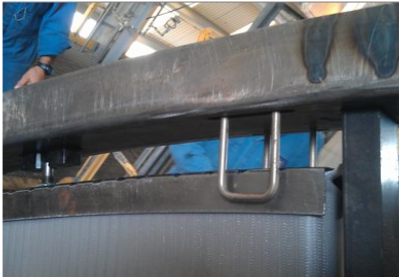
Figure 4. Fixation of segment to the rim via clamp springs (during test operation).
