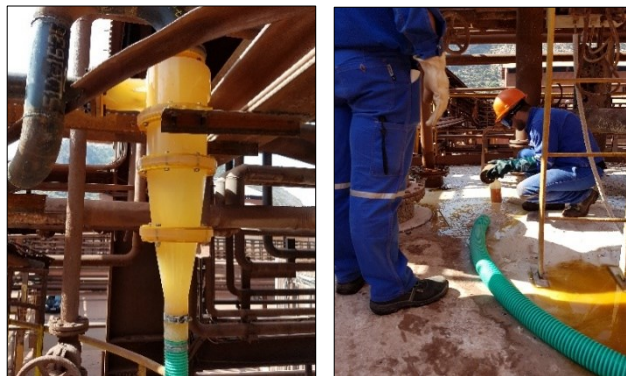
Figure 8. (a) Test hydrocyclone on site; (b) Sampling whilst the test run.
