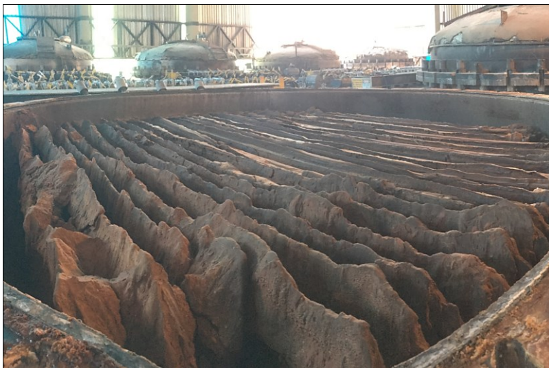
Figure 1. Scale on top of the pressure leaf filter before filter bag refurbishing.
