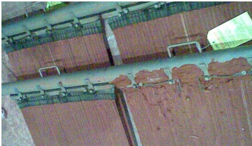
Figure 17. Effect of Sefar x-Scale EPDM closure on scaling.
