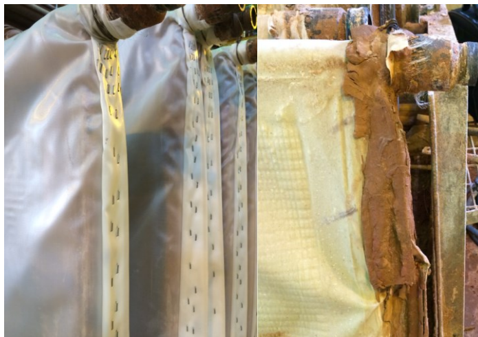
Figure 15. Regular leaf filter closing by stapling, before and after use.
