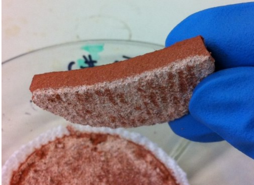
Figure 3. Formed dried filter cake showing a layer of TCA particles (white) and a layer of bauxite residue particles (red) above it.
