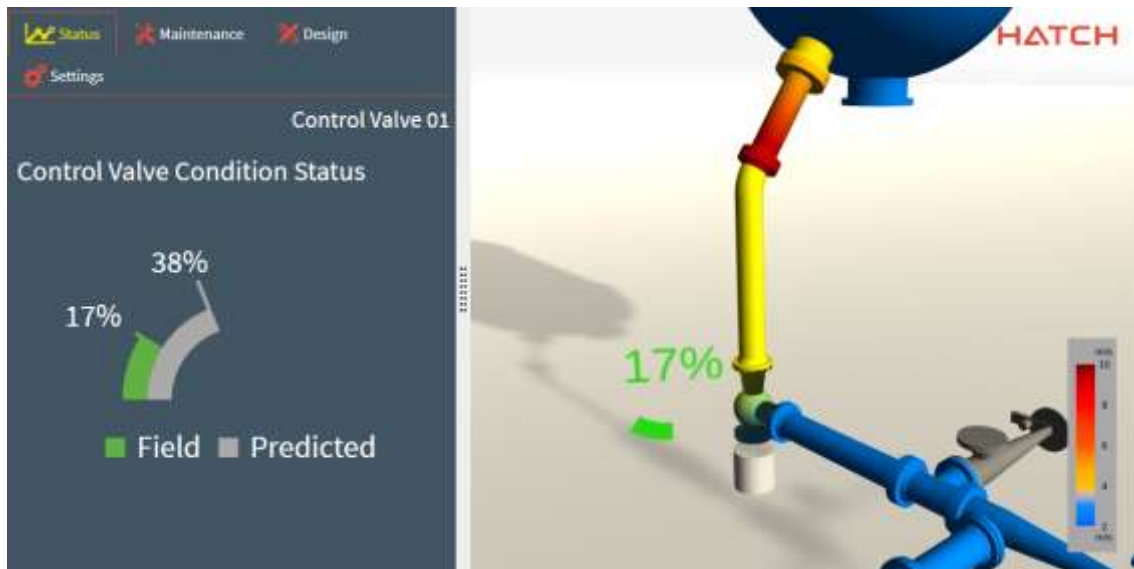
Figure 10. Condition monitoring of control valve, calculated vs feedback position.
