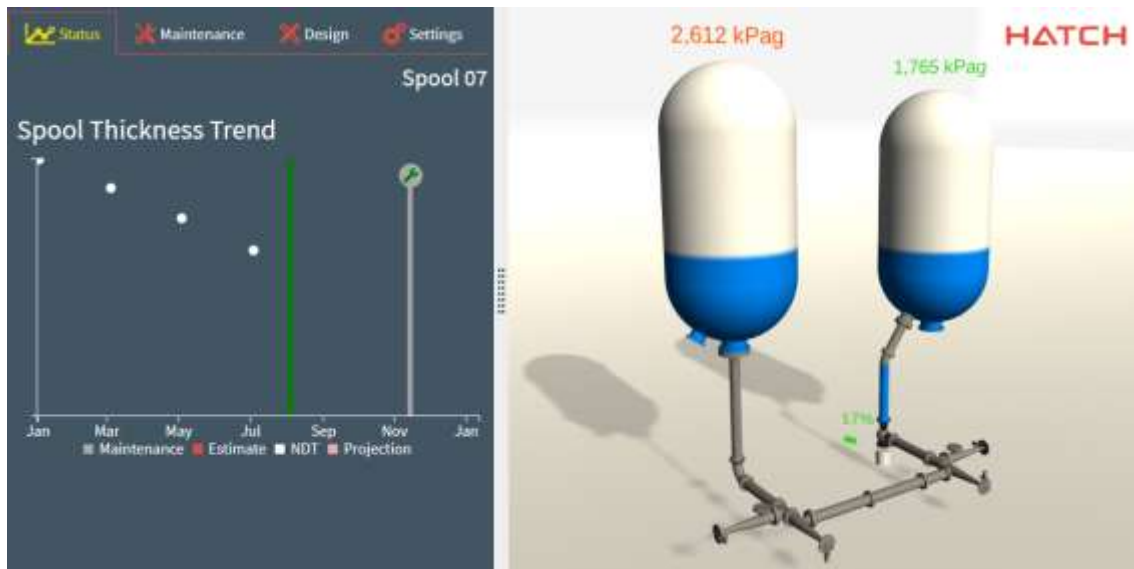
Figure 6. Chart displaying NDT data for selected piping spool.
