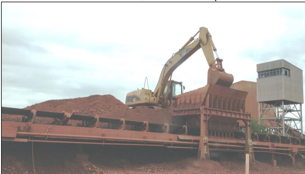
Figure 3. Excavator adding bauxite directly to conveyor belt.
