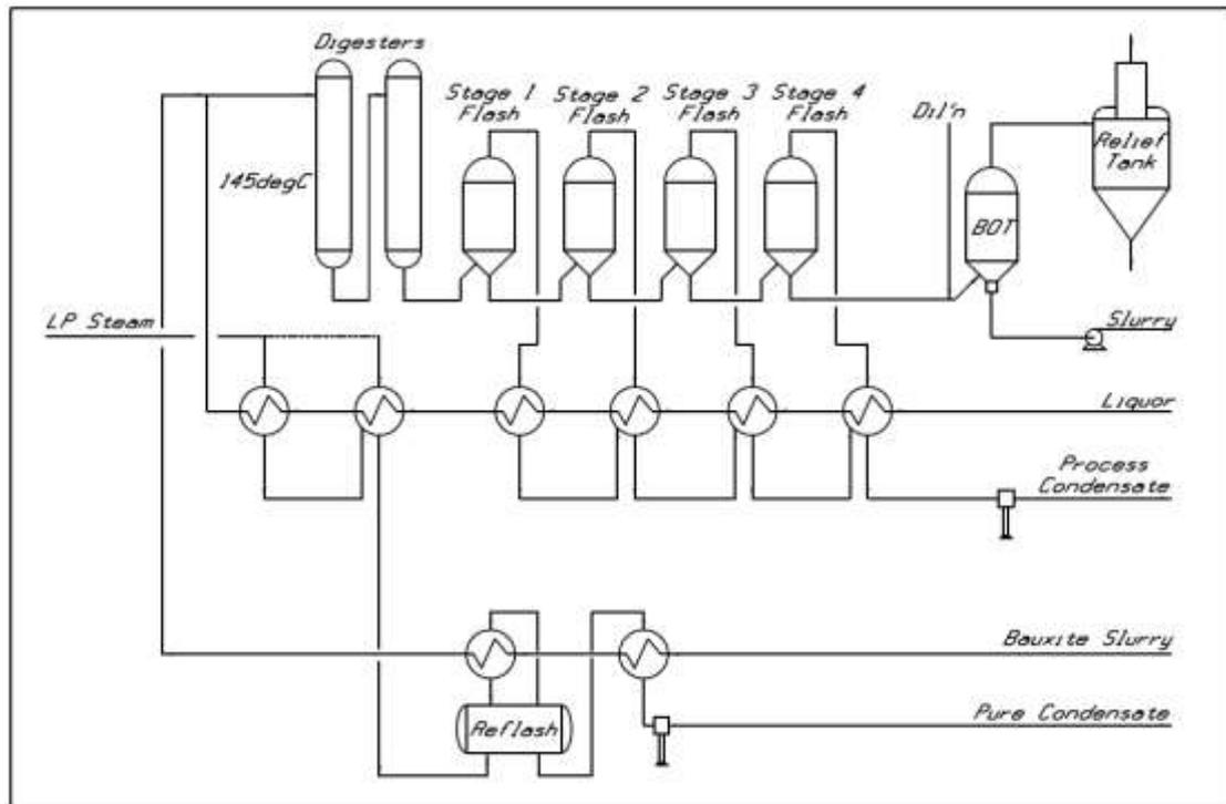
**Figure 1. Dual stream low temperature digestion flowsheet.**
