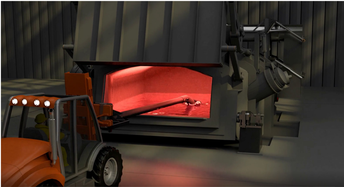
Figure 12. Stirring process with wheel loader.
