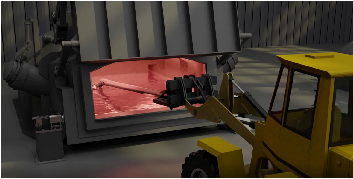
Figure 11. Stirring process with wheel loader.
