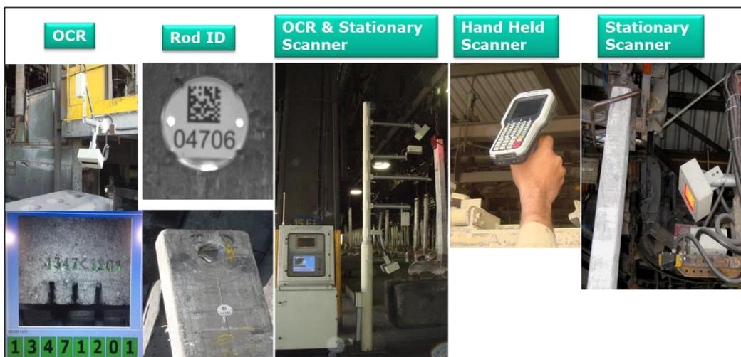
**Figure 1. Rod and Anode Tracking Information System hardware.**
