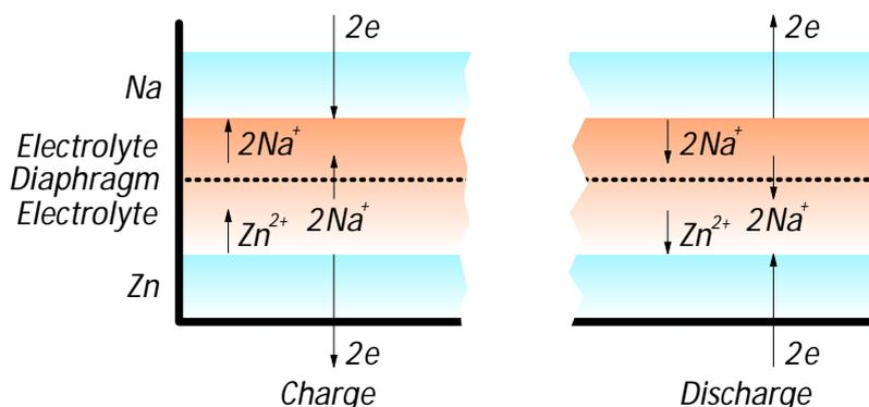
Figure 1. Principle of the liquid metal battery.
