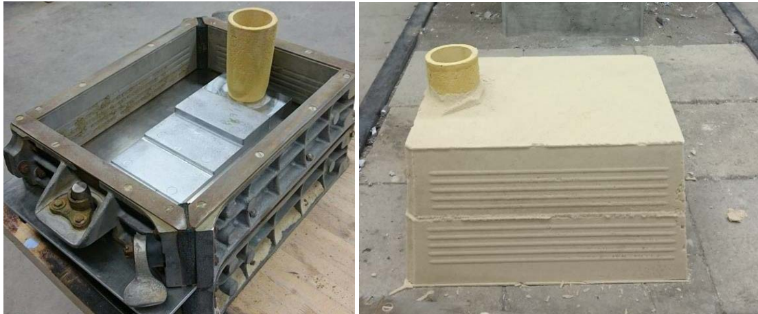
Figure 2. Step casting model with Kalpur filter cup – Mold before pouring.
