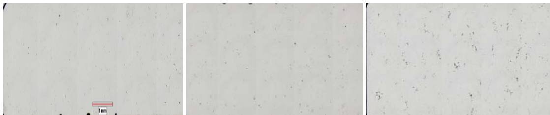
Figure 6. Mosaic in the 6 mm, 13 mm and 25 mm of the degassed A206 step casting.
