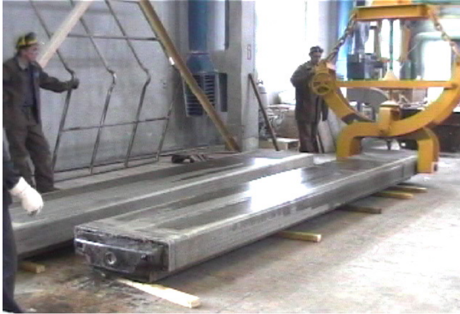
Figure 6. Magnesium T-bar Cast using Hatch Hot Top Technology.
