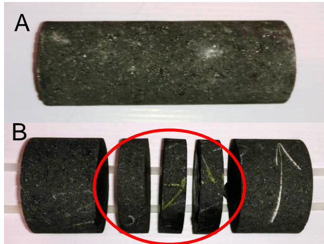
Figure 3. Anode core shapes for measurement of electrical resistivity using standard method (A), and Van der Pauw method (B)
