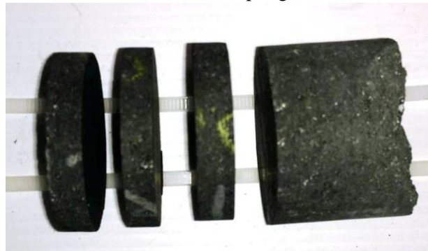
Figure 4. Broken sample prepared for measurement using Van der Pauw method.
