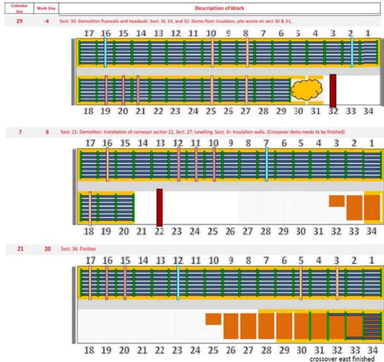
Figure 2. Different demolition and installation tasks and sequences
