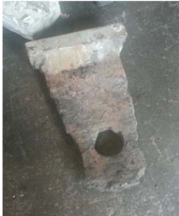
Figure 13. Strong copper tab oxidation in D18 Technology.
