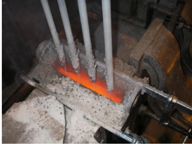
Figure 4. ESW welding system – view from the top showing the molten slag.
