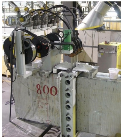
Figure 6. ESW welding equipment.
