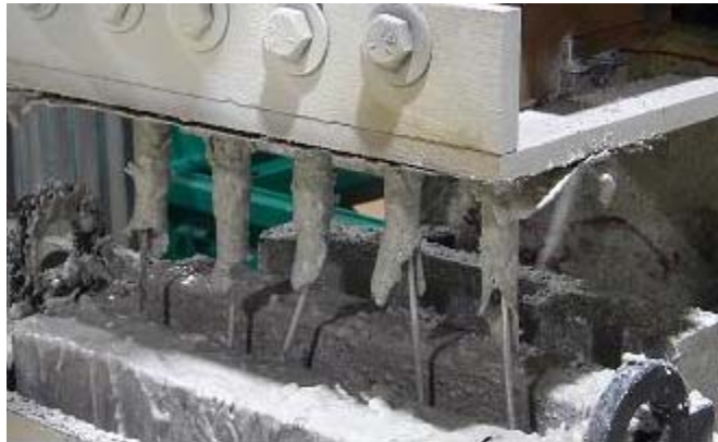
Figure 5. Consumable guides and electrode wires.
