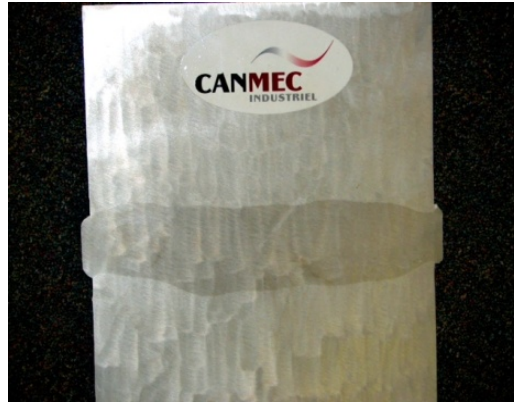
Figure 10. Electroslag weld macroetch.
