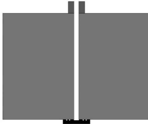
Figure 3. Bus bar assembly before using ESW.
