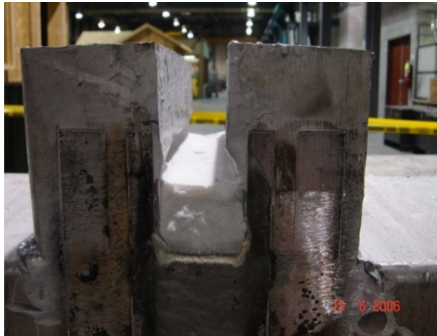
Figure 9. ESW joint showing the solidified slag.
