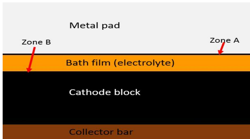
Figure 2.2. Sketch of the interfaces and zones at the carbon cathode from [2].
