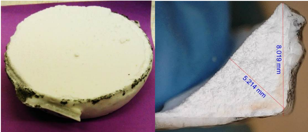
Figure 1. Left: Photo of alumina disc after recovery from the bath, Right: Microscope photo of the cross section of the edge (series A, secondary alumina, 30 s)
