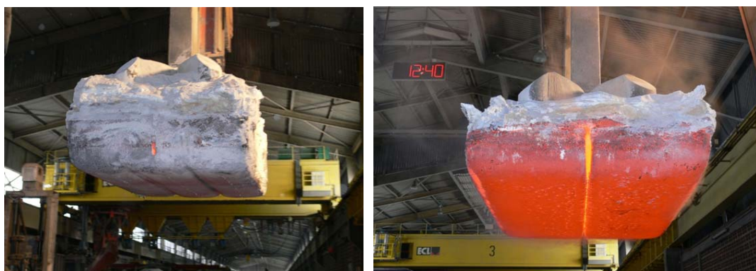
Figure 10. Consumption of anode with three slots as a function of time in the cell.
