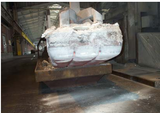
a. Anode after 33 shifts in the cell.
