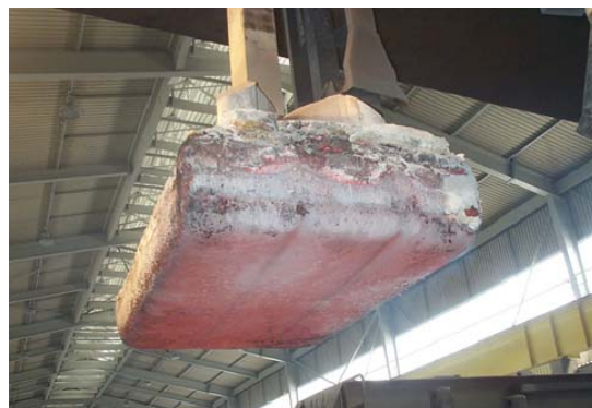
b. Anode after 44 shifts in the cell.
