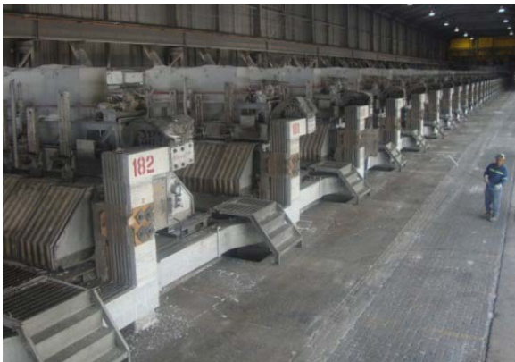
Figure 1. D18 Technology cells in Potline 1.
