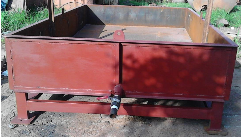
Figure 3. Experimental cell for investigation of oxalate degradation rate by solar radiation.
