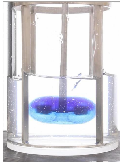
Figure 10. Thick Carbopol solution yield stress 33 Pa at 400rpm. [5]
