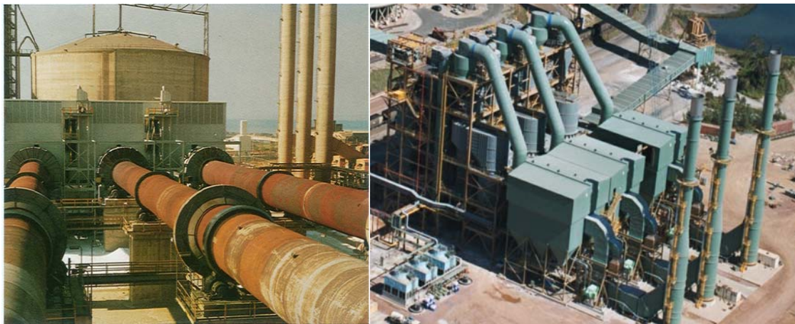
Figure 1. 3x \text{Ø} 3.95 \times 107 \text{ m} rotary kilns 3 x 4500TPD GSC units with bag filters.
