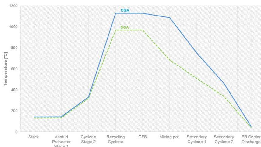
Figure 4. Temperature profile of SGA and ceramic grade alumina CGA.
