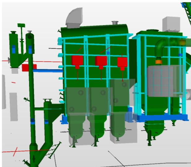
**Figure 6. The purpose designed fluid bed cooler, capable to operate at two very different modes.**
