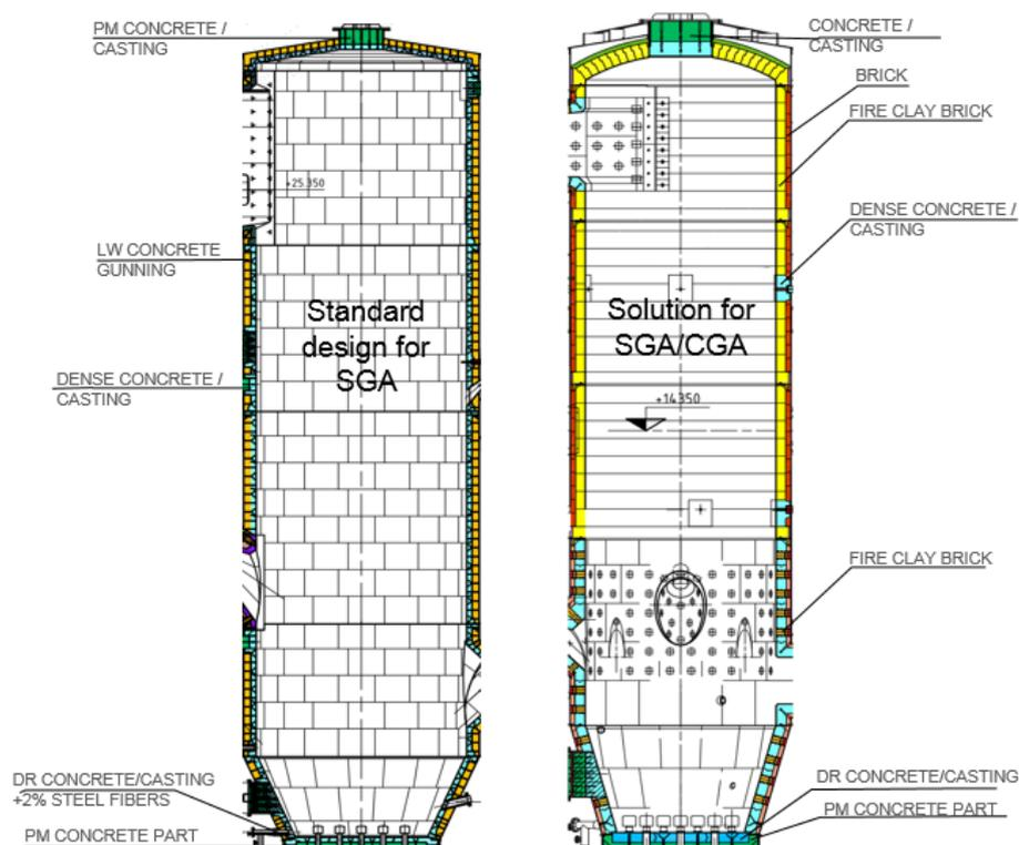
Figure 7. Refractory design for “standard” furnace used for SGA production (left) and new design for the dual purpose calciner (right).
