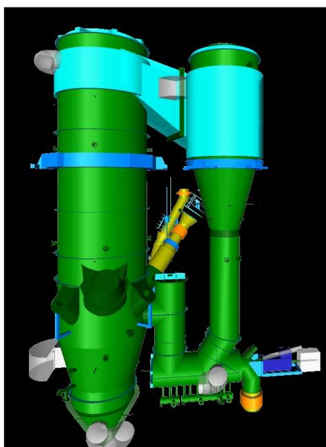
Figure 5. Model of the CFB furnace group for the dual purpose calciner. The use of a ramp design in the recycle cyclone eliminated the need for a vortex finder.
