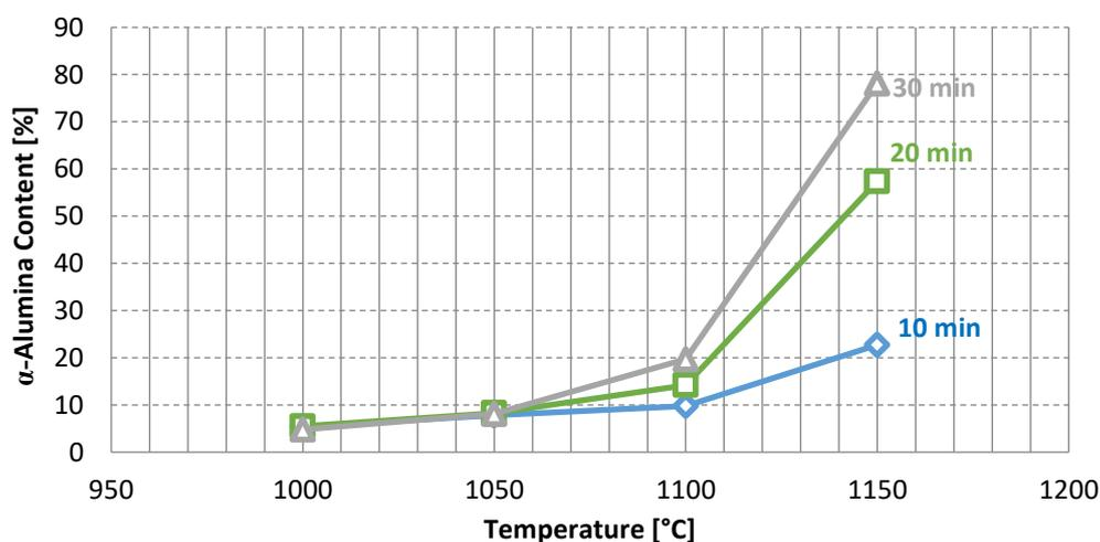
Figure 2. Alpha alumina content vs. Temperature.
